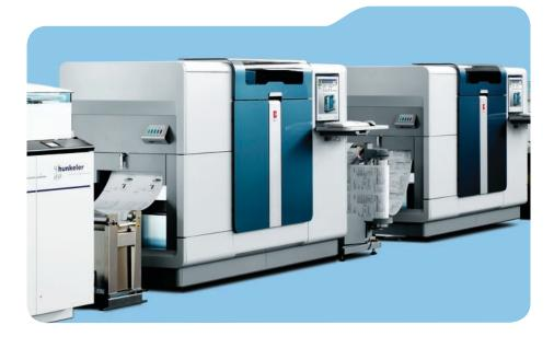
and Graphic Arts applications converge and TransPromo documents gain momentum. State-of-the-art LED imaging technology produces output with enhanced print and image quality, while Super Cell technology enables printing of 256 grayscales. The result? A system ideally equipped to address your most exacting requirements – today and tomorrow.
